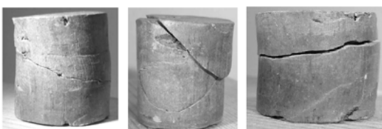
Figure 5: Macroscopic observations of cracks on boom clay samples under desaturation
