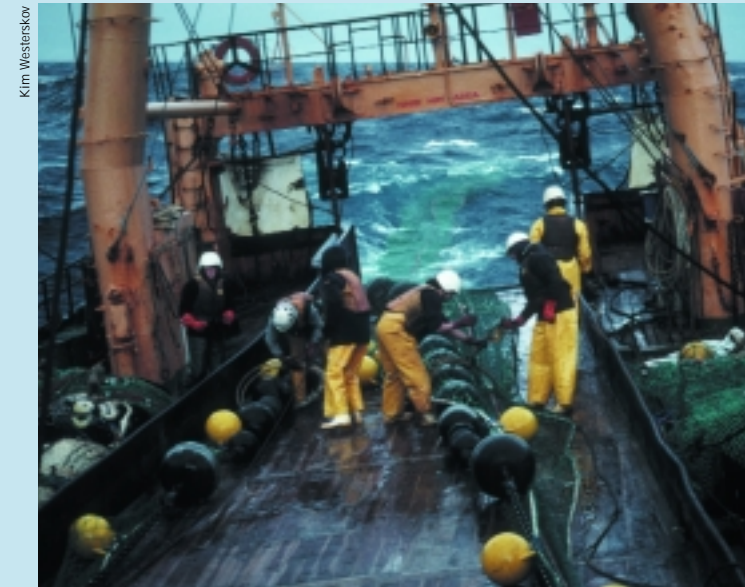
Orange roughy fishermen offloading the steel rollers that weigh down bottom trawl nets.
