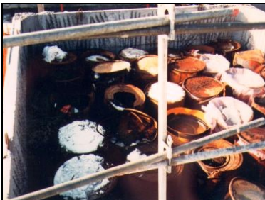
Damaged and leaking waste barrels inside CSM
