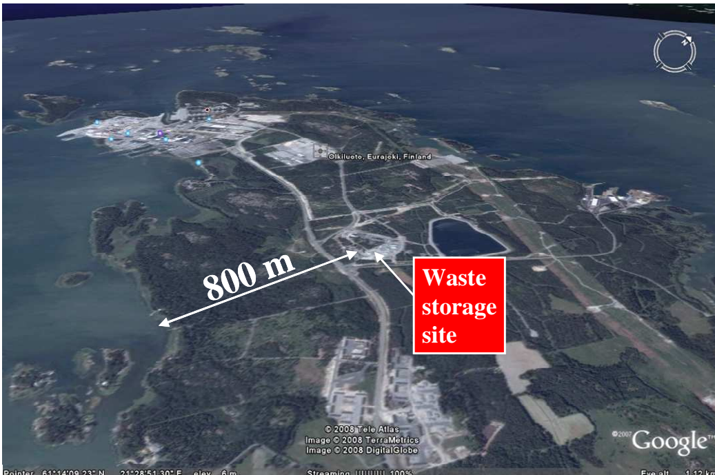
Figures 1 and 2: The proposed waste depository in Olkiluoto is located less than a kilometer from the Baltic sea, in a place where the groundwater flows from the bedrock directly into the sea.
