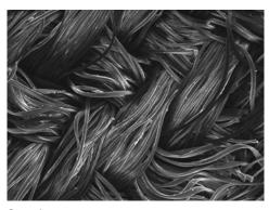
Sample 1: SympaTex $^{\circ}$  finish at a magnification of 130 Illustration 2 – fabric with finish
