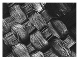
Sample 2: Schoeller Ecorepel<sup>®</sup> at a magnification of 130 Illustration 1 – fabric with finish
