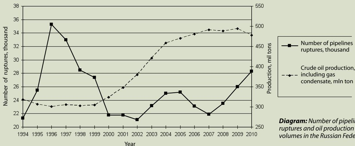
**Diagram:** Number of pipelines ruptures and oil production volumes in the Russian Federation.
