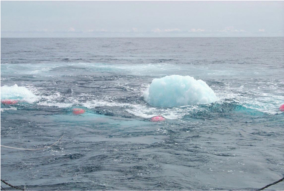
An airgun array being fired during a marine geophysics research project off the coast of Nicaragua
