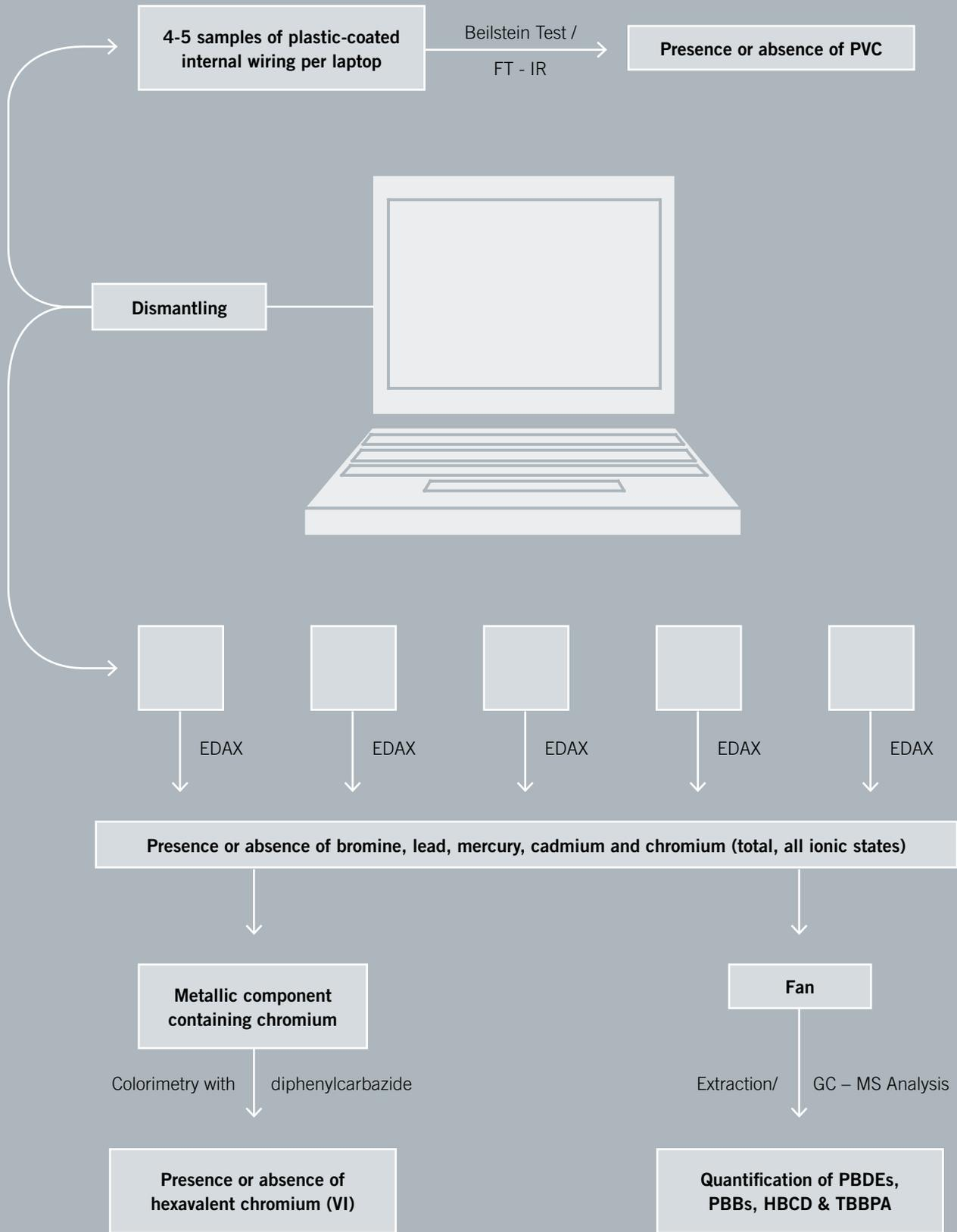
Figure 1. Dismantling of the laptop's components and their analysis
