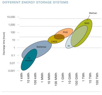
FIGURE 10.33 | OVERVIEW STORAGE CAPACITY OF
