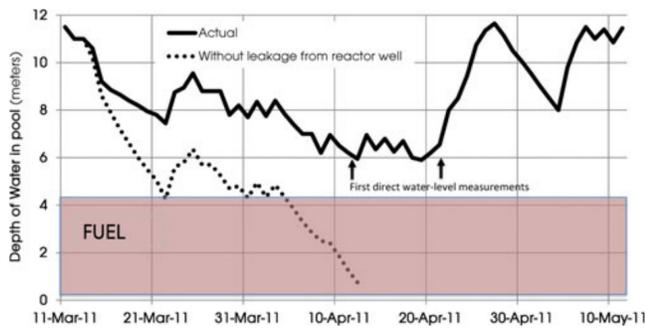
**Figure 2.** Solid line: TEPCO reconstruction of the history of the water level in pool 4 during the two months after the earthquake.<sup>21</sup> The arrows show the first actual measurements, the first of which was made on 12 April and the second on 22 April. The dotted line below shows an estimate in the National Academy of Sciences report of the amount of water that would have been in the pool in the absence of water leaking into the pool from the adjacent reactor well.<sup>22</sup>
