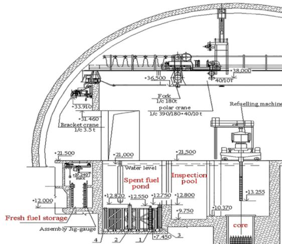
VVER-1000/320 reactor containment showing location of spent fuel pool (source<sup>16</sup>)
