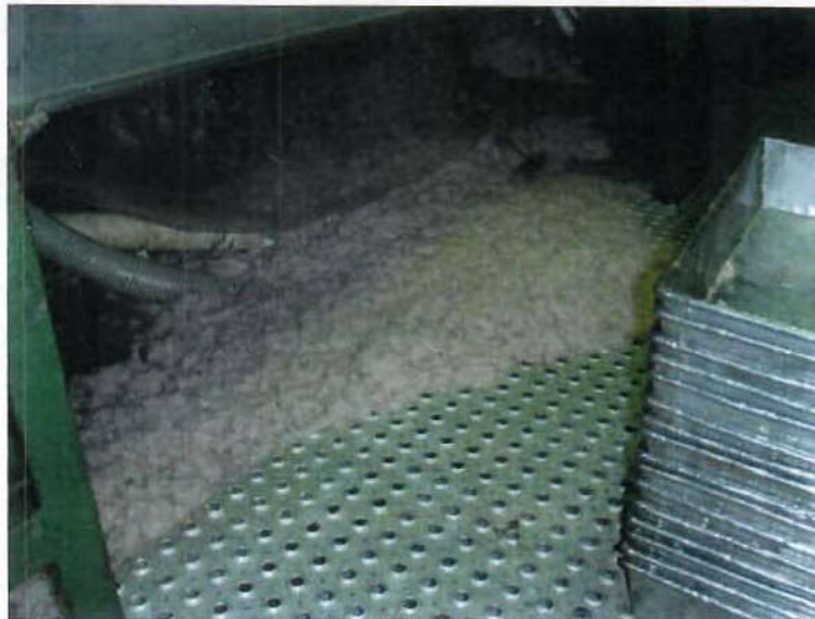
Figure 10a – SBW being lost from Surimi refining process on the Tomi Maru 87
