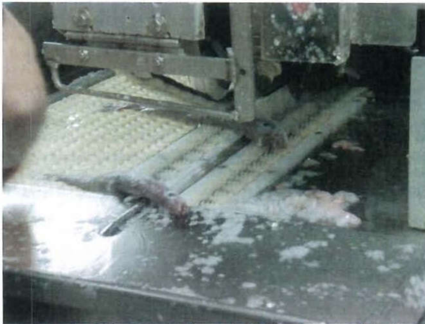
Figure 6 – Baader 424 Processing Machine – the gill plate of the fish is hooked over the alignment lug and carried through the saw by the transport belt, a secondary spring-loaded belt presses down on top of the fish as it is carried through the saw.
