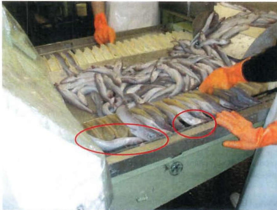
Figure 4 – Loading fish into the Ira 110. Precise placement of fish into the trays is critical for achieving compliant cuts. Fish circled in red will produce non compliant cuts.
