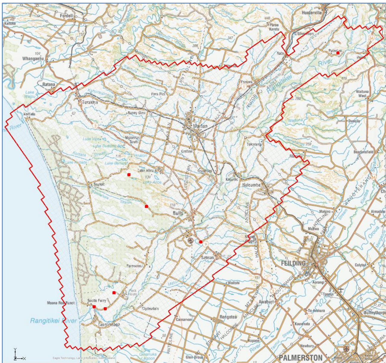
Figure C-4. Wells (groundwater abstraction bores) and well (WEL) cells in Layer 4 in the model (red squares).
