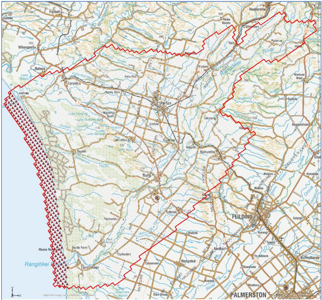
Figure 4-12. General Head Boundary (GHB) cells in Layers 1–6 in the model (brown triangles).
