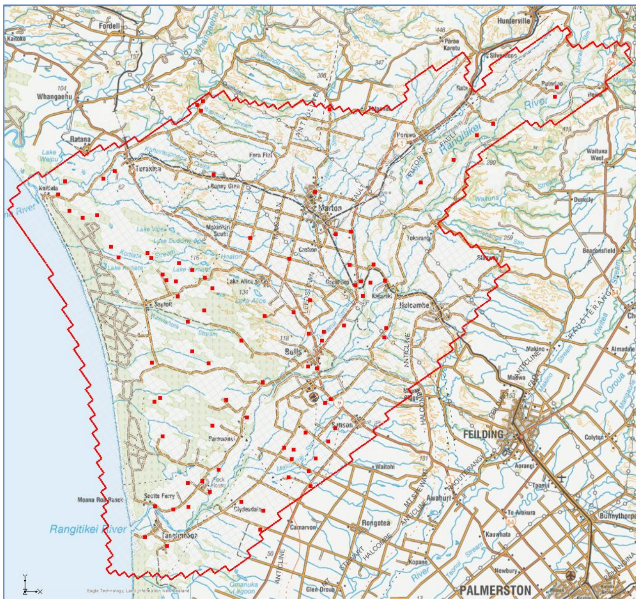
Figure 4-17. Wells (groundwater abstraction bores) and well (WEL) cells in Layers 1–8, 10 and 11 in the model (red squares). There are no wells in Layer 9. Wells in different layers are presented in Appendix C.
