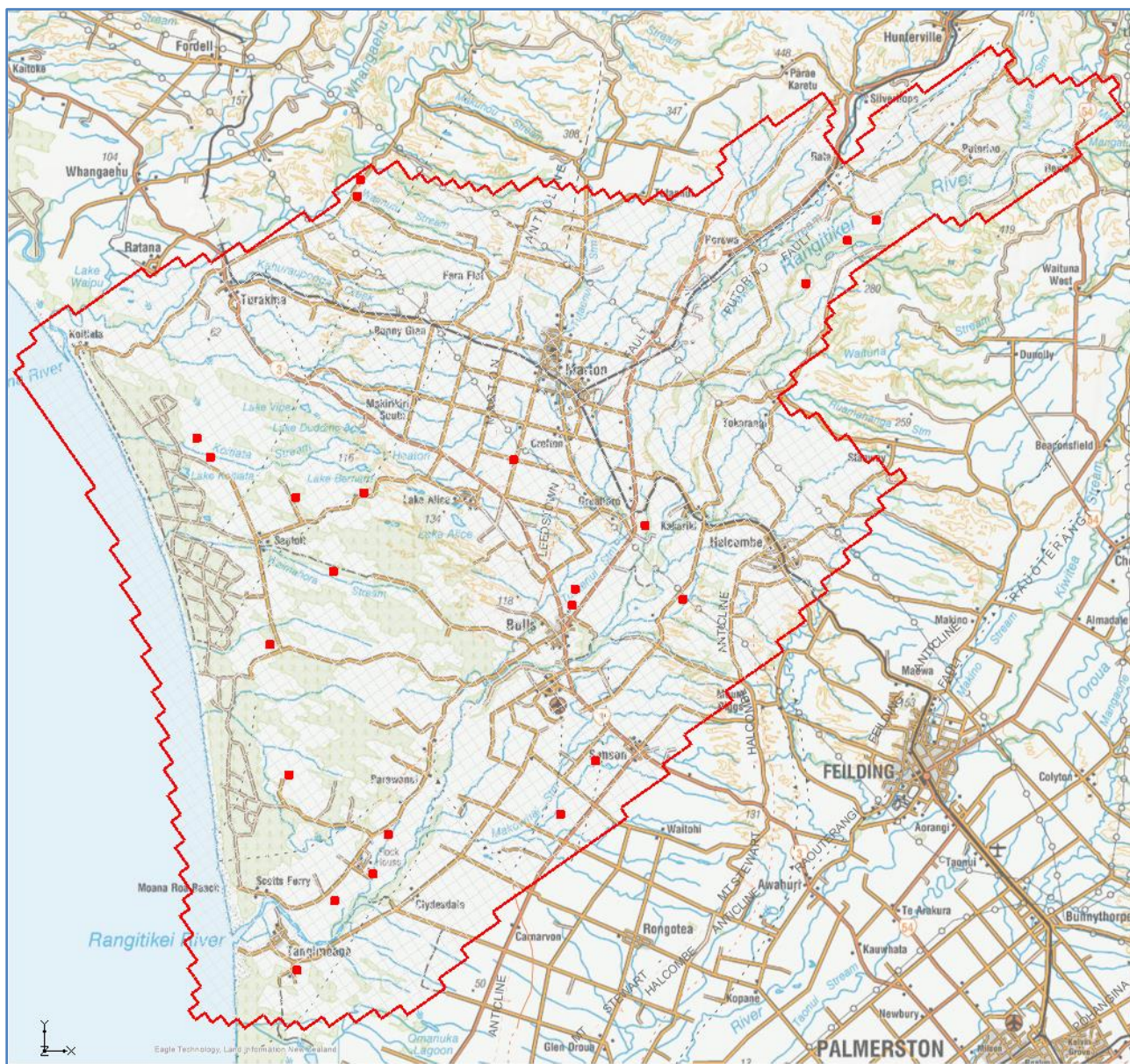
Figure C-6. Wells (groundwater abstraction bores) and well (WEL) cells in Layer 6 in the model (red squares).
