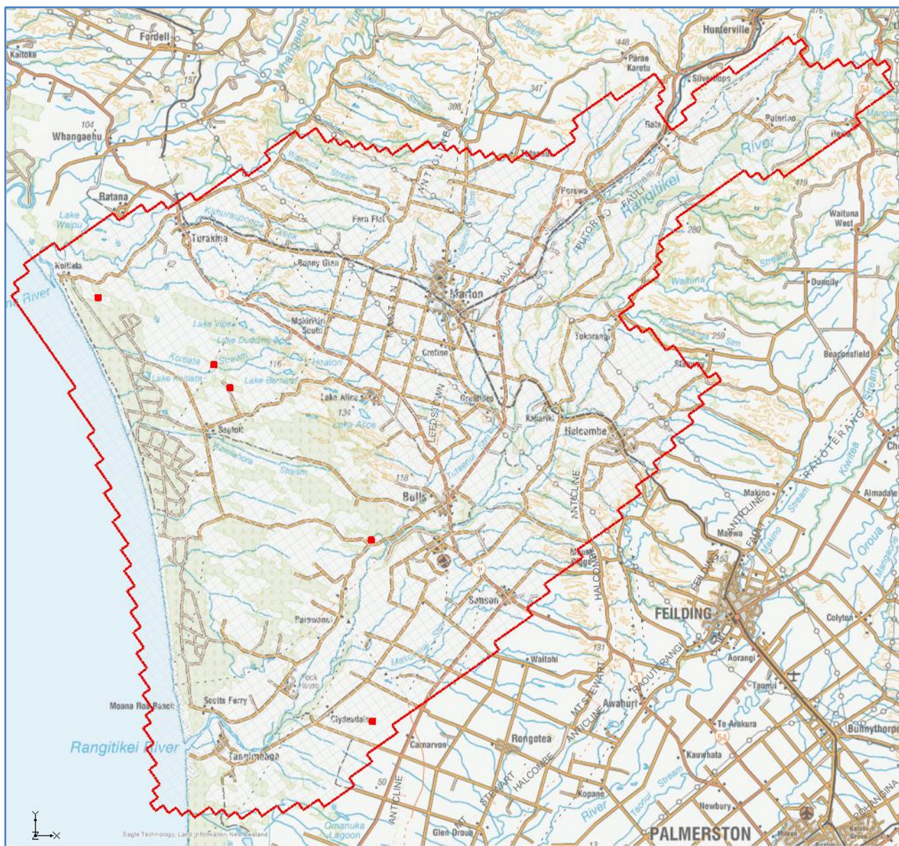
Figure C-9. Wells (groundwater abstraction bores) and well (WEL) cells in Layer 10 in the model (red squares).
