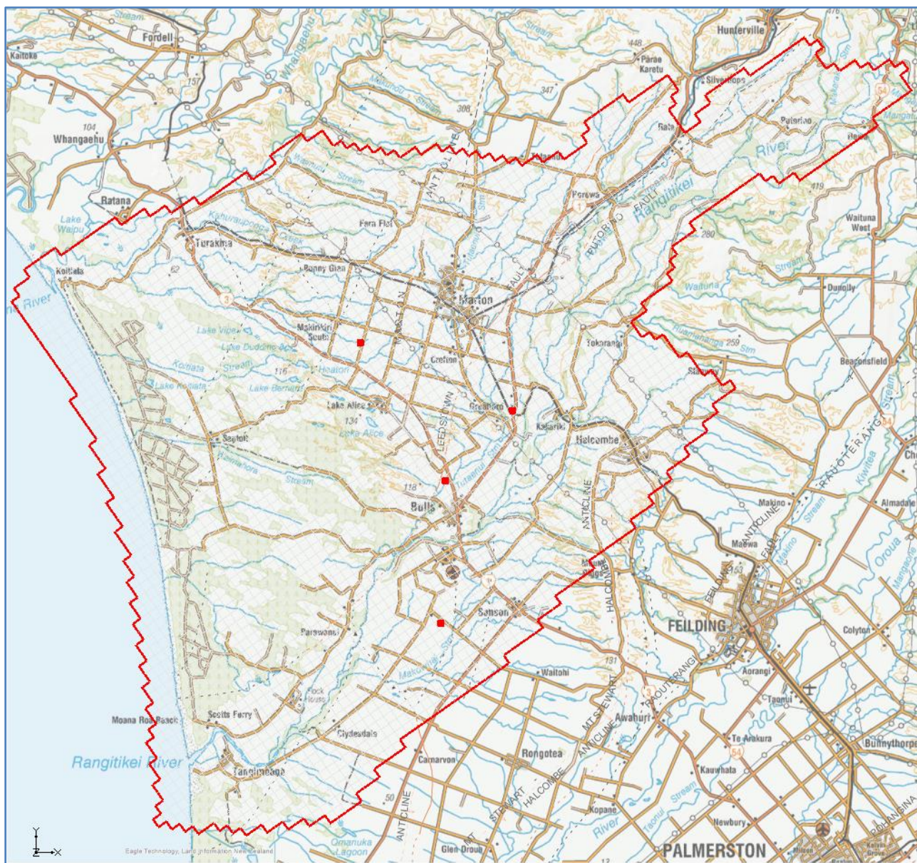
Figure C-1. Wells (groundwater abstraction bores) and well (WEL) cells in Layer 1 in the model (red squares).
