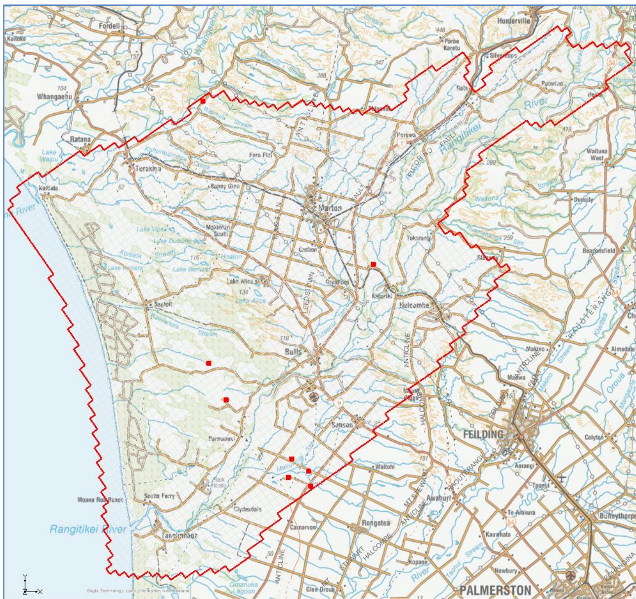
Figure C-7. Wells (groundwater abstraction bores) and well (WEL) cells in Layer 7 in the model (red squares).
