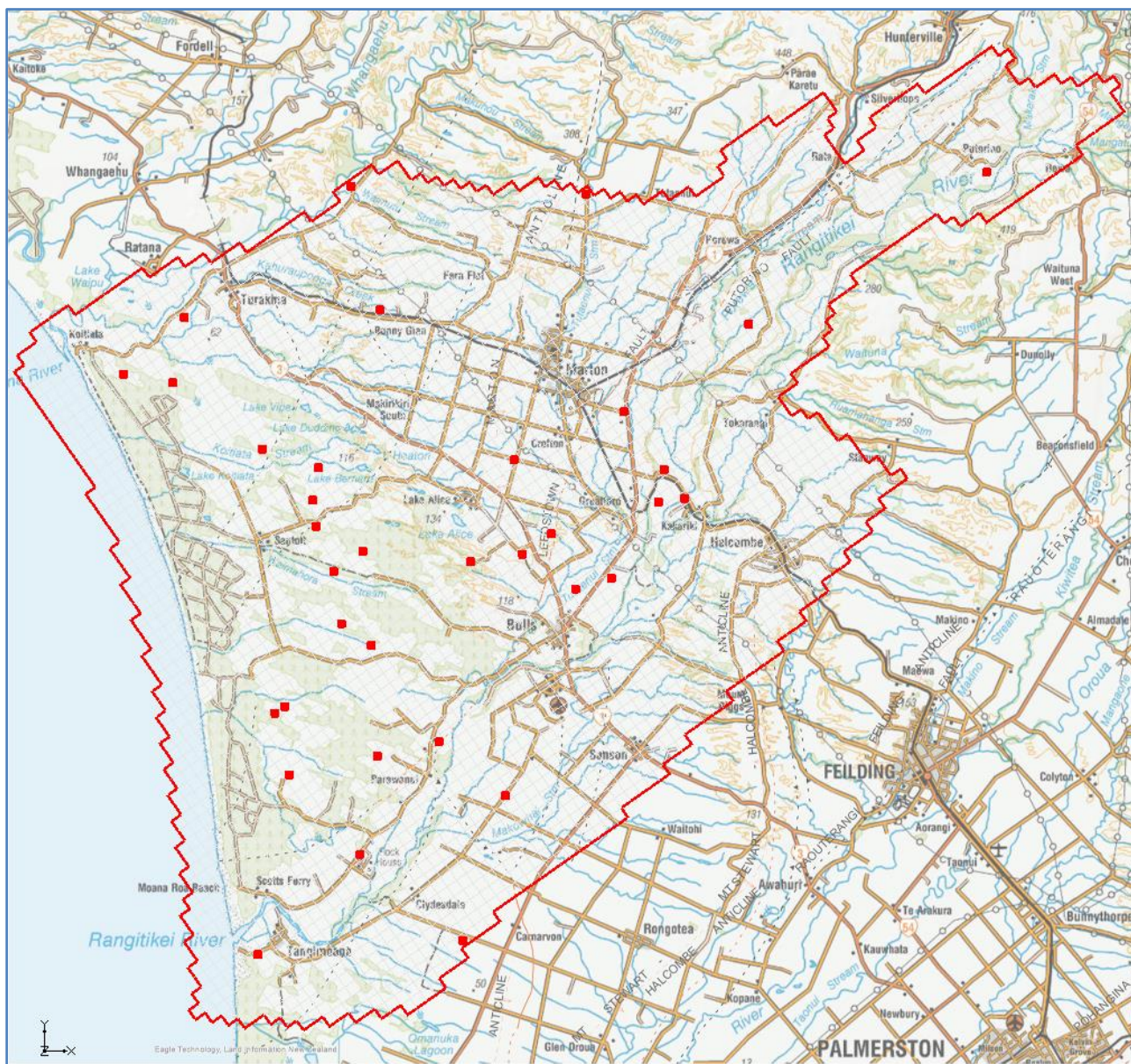
Figure C-5. Wells (groundwater abstraction bores) and well (WEL) cells in Layer 5 in the model (red squares).
