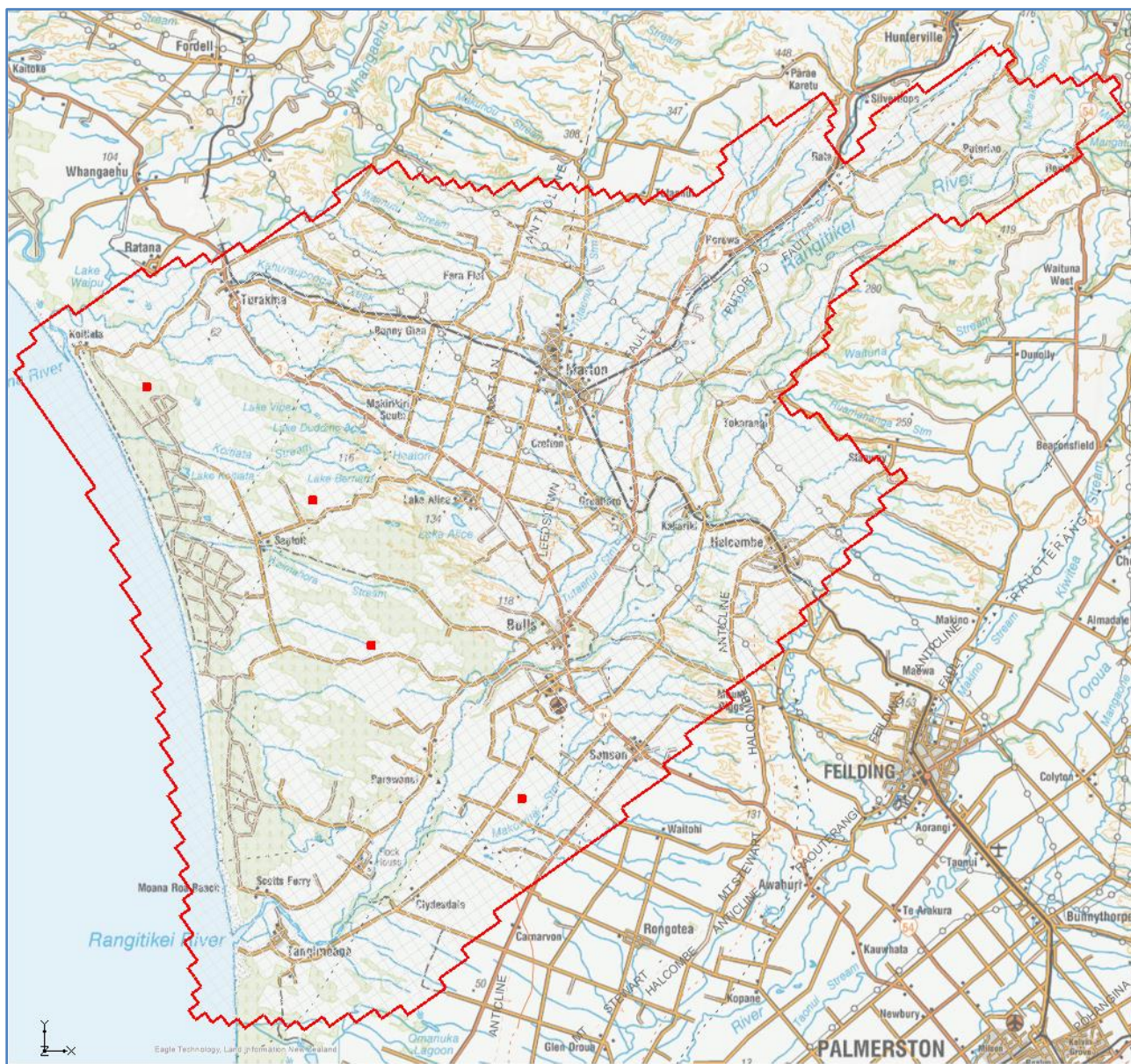
Figure C-10. Wells (groundwater abstraction bores) and well (WEL) cells in Layer 11 in the model (red squares).
