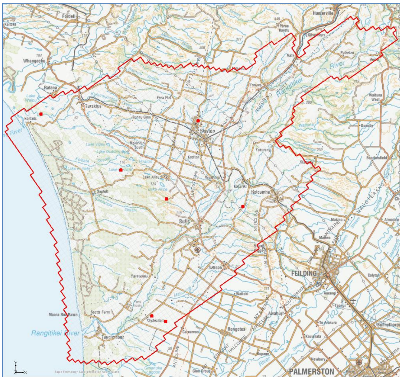
Figure C-8. Wells (groundwater abstraction bores) and well (WEL) cells in Layer 8 in the model (red squares).
