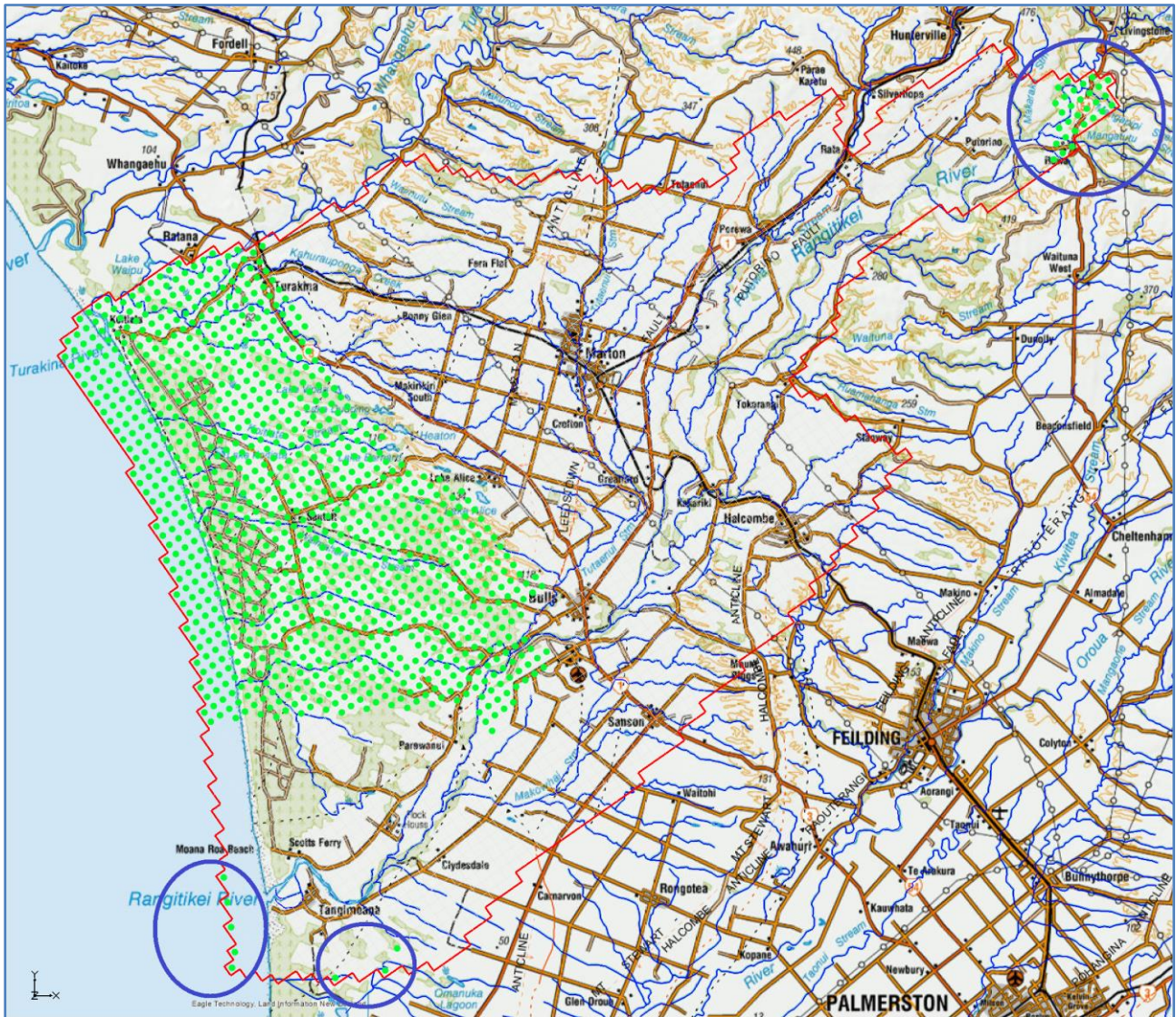
Figure 4-16. Rivers and streams in the area (blue lines) and drain (DRN) cells in Layer 1 in the model (green dots). The blue circles mark likely inappropriate designation of DRN cells. Not the inappropriate offshore assignment of drain cells.
