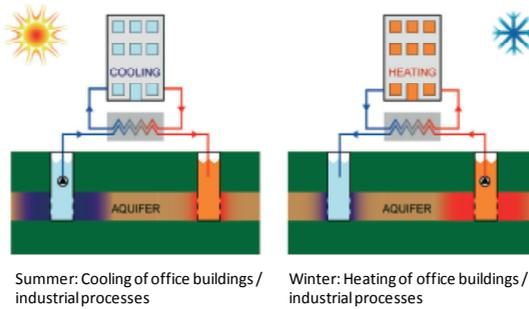
Figure 2 – Layout Scheme of an Aquifer Storage System
