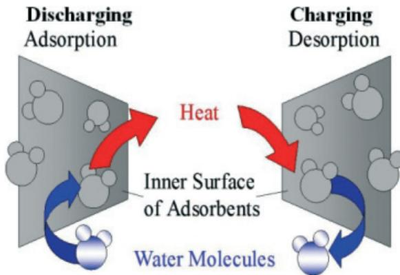
*Figure 5 – TES De/Adsorption Process*
