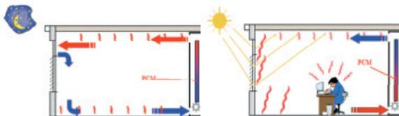
Figure 4 – Layout Scheme for “Passive Cooling”
