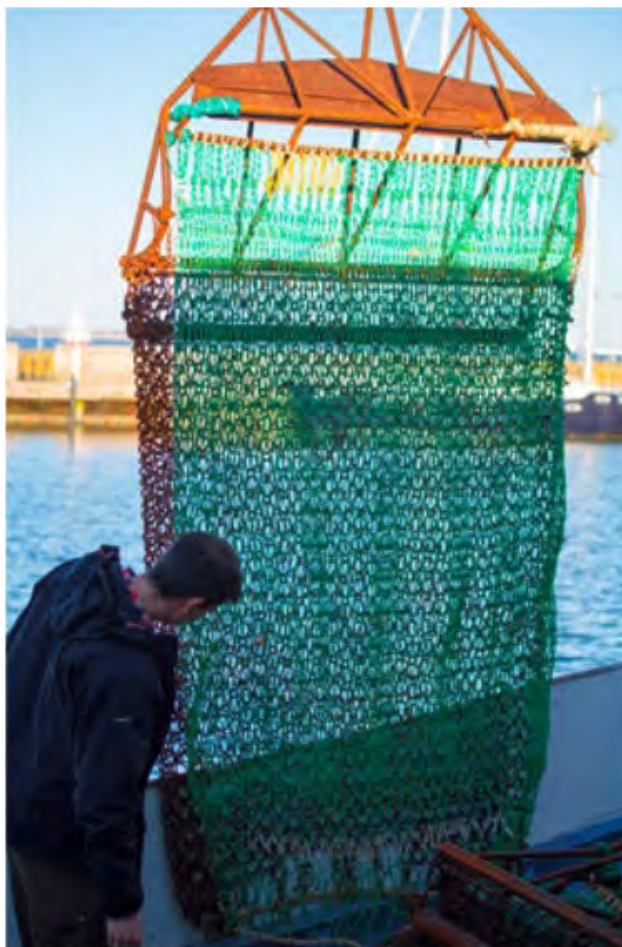
Figure 6. Commercial lightweight mussel dredge used in the Limfjord. (Photo credit: Chris Grieve)
