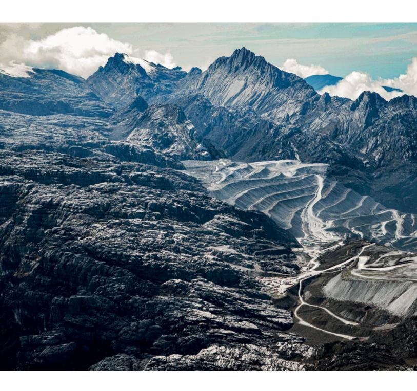
The inevitable result of Freeport Indonesia hollowing out Nemangkawi mountain through open pit and underground mining is a massive amount of waste rock that needs to be placed somewhere. Here it has been trucked into a ziggurat of mine waste just a few kilometers from a glacier, creating a serious risk of acid mine drainage from oxidation of sulfide minerals, a problem that can mobilise toxic heavy metals and that could persist for many decades after the gold has run out. (27/03/2013).
