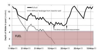
**Figure 2.** Solid line: TEPCO reconstruction of the history of the water level in pool 4 during the two months after the earthquake.<sup>21</sup> The arrows show the first actual measurements, the first of which was made on 12 April and the second on 22 April. The dotted line below shows an estimate in the National Academy of Sciences report of the amount of water that would have been in the pool in the absence of water leaking into the pool from the adjacent reactor well.<sup>22</sup>
