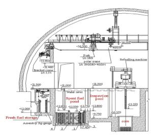
VVER-1000/320 reactor containment showing location of spent fuel pool (source<sup>16</sup>)
