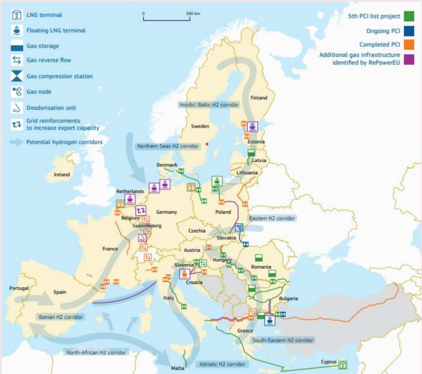
Figure 4: European map of infrastructure for gas – PCIs and additional projects identified through REPowerEU, including hydrogen corridors.
