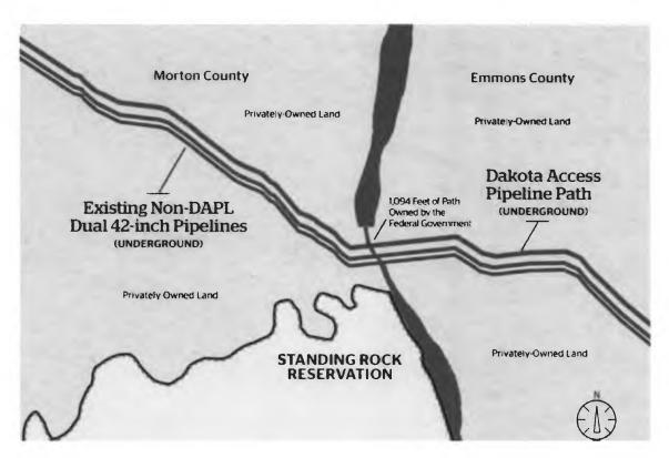
[¶31] As depicted in the image below, the pipeline "crosses" 90 to 115 feet beneath Lake Oahe along the route of an existing pipeline — the Northern Border Pipeline. Plaintiffs selected this crossing location because it would traverse a path that was already disturbed by existing infrastructure, thus reducing the risk of any negative impact to historic resources or cultural features.
