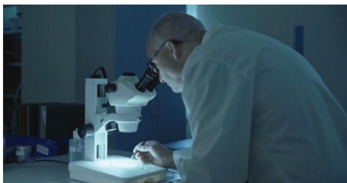
Greenpeace scientist Dr David Santillo examining the surface of a silver filter used to collect a sample of particles from the air, prior to analysis of the sample for the presence of microplastics using an infrared microscope system. Photo ©Jack Taylor
