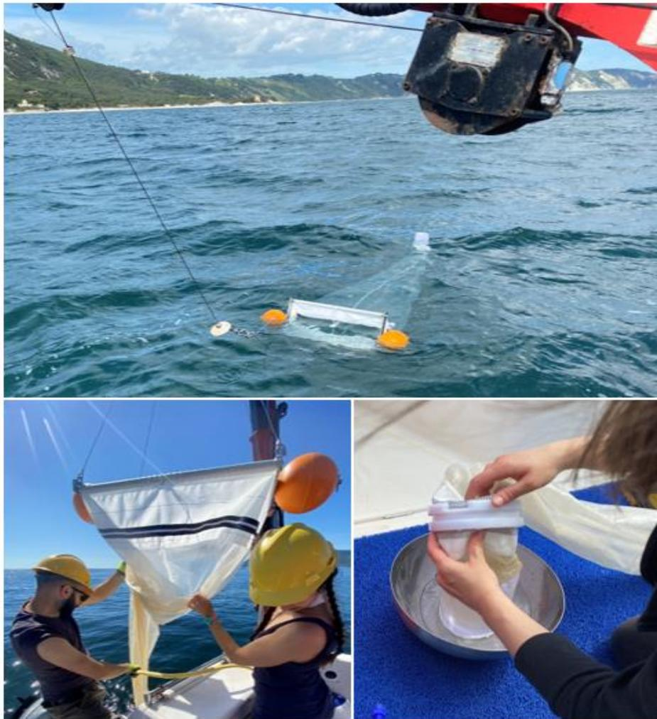
**Fig. 3** Monitoring the occurrence of microplastics in the first 15-25 cm of surface water layer using a Manta trawl. Sampling performed in May 2020, operating transects in several stations located along the Conero Riviera (Ancona coast, Marche, Italy).
