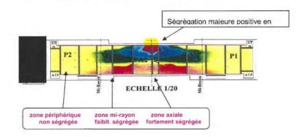
FIGURE 5: PLAQUE TUBULAIRE 1300 MWE - CARTOGRAPHIE DE CARBONE
