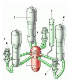
FIGURE 3 REACTOR N1 PRIMARY COOLANT CIRCUIT TYPICAL OF 3-LOOP 900 MWe SERIES
