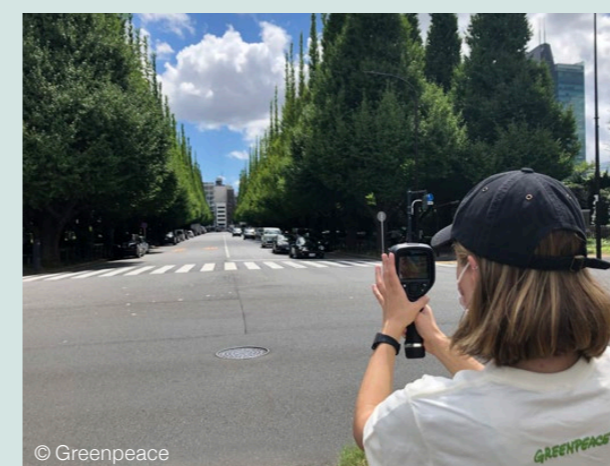
Measuring the surface temperatures
