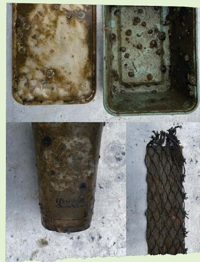
▲ Picture 3: Product samples were submerged in the sea before cleaning
