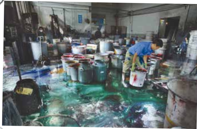
images: (1) A dyeing plant in Shaoxing, Zhejiang; (2) A dyeing factory in Shaoxing Binhai Industrial Zone: a plant with 5 dyeing machines will need about 250kg of dyestuff. Along with other additives, about 2,500kg of dyestuff paste circulates in the plant every day. Images © Qiu Bo / Greenpeace
