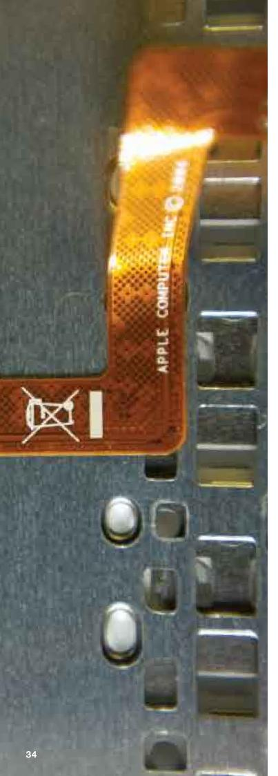
Of the three mouse touchpads (#01) analysed, extractable BFRs were identified in only the component from the Apple laptop (LTOP09). PBDEs were present at low levels in this sample, including deca-BDE (BDE-209) at 12.2 mg/kg and nona-BDEs at 1.87 mg/kg. This component also contained the brominated chemical TBBPA at a higher concentration of 125 mg/kg.
