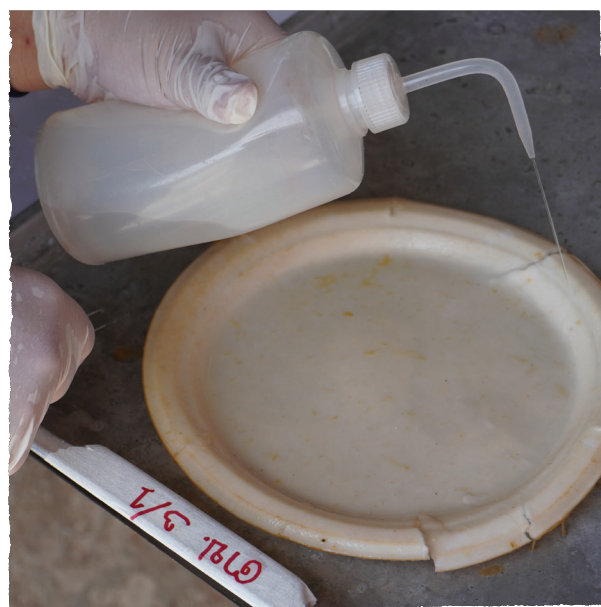
Researchers used distilled water to wash out any residues from the product for examination to assess the presence of microplastics.
