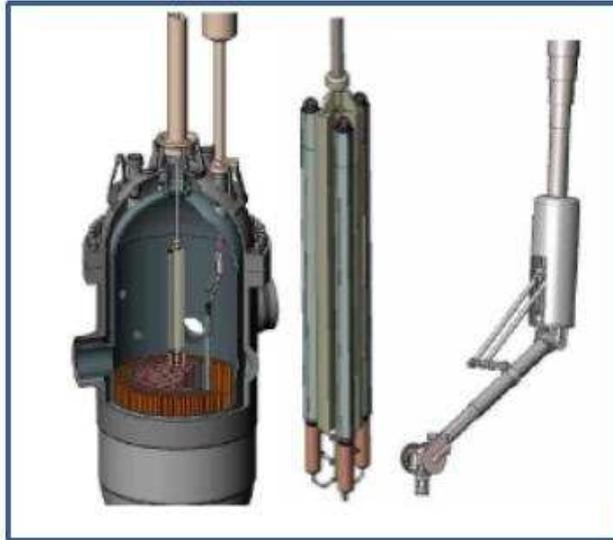
Figure 23: Handling arm and transfer cask (reference 64)
