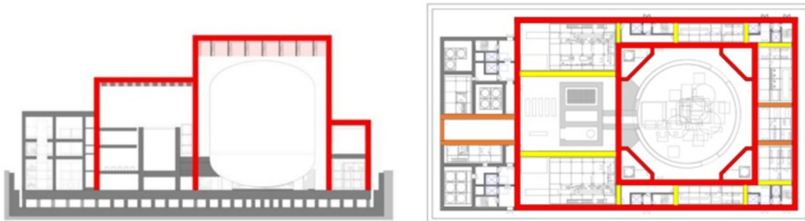
Figure 6: Extent of hazard shield shown in red (elevation on left (l), plan on right (r)) (ONR 2024c)
