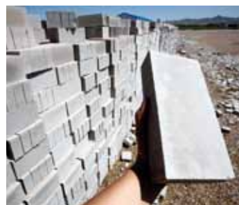
June 2010. Bricks made from coal ash at the Yuanbaoshan Power Plant, Inner Mongolia. © Zhao Gang/Greenpeace
