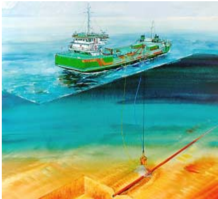
Fig. 18: Jet trenching with mass flow excavation
