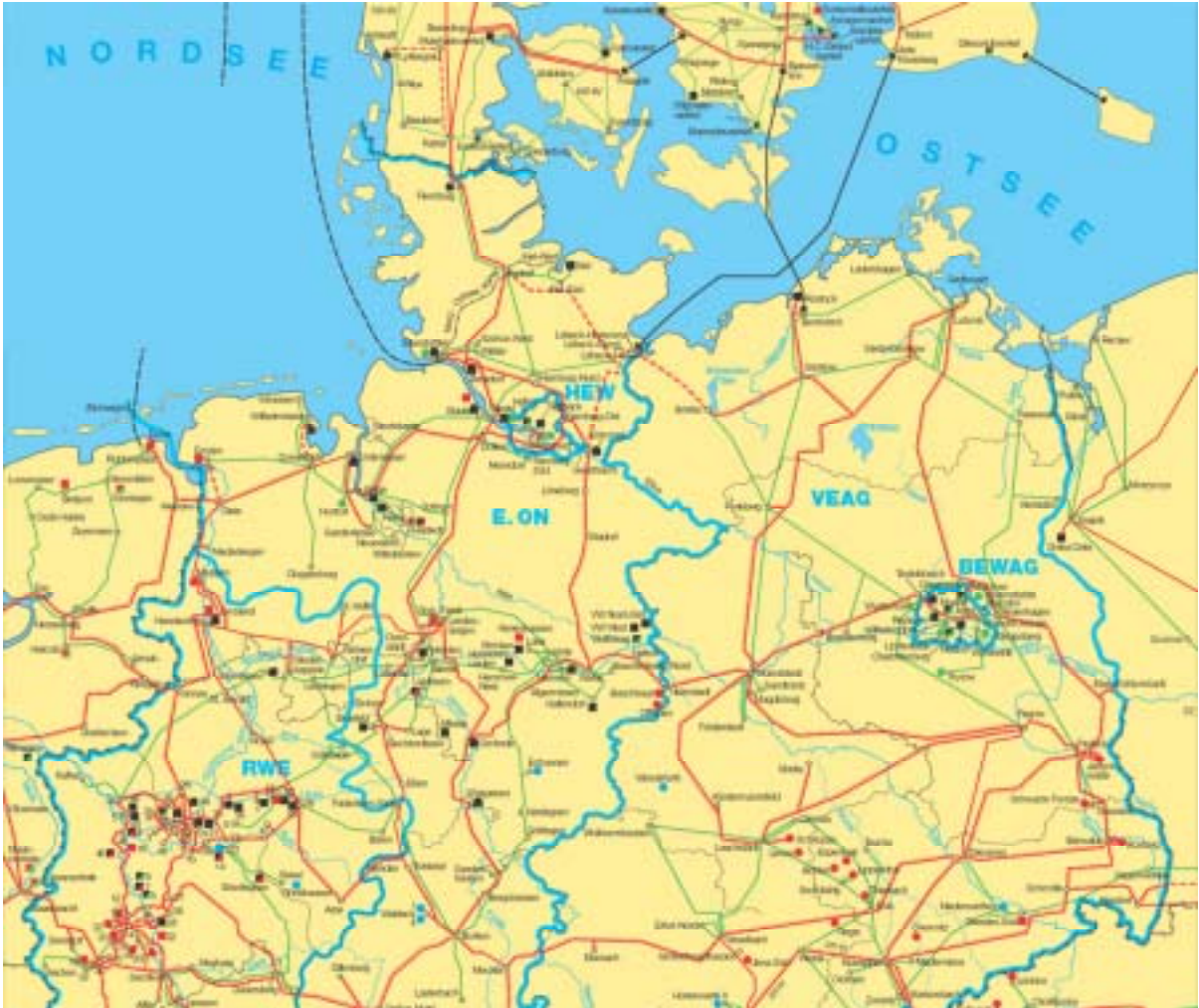
Fig. 6: Electrical transport network in northern Germany [Ref 49]. The red lines indicate the 380kV grid, the green lines the 220kV grid. The small open circles indicate grid nodes. The black and coloured squares and the larger coloured dots indicate power plants.
