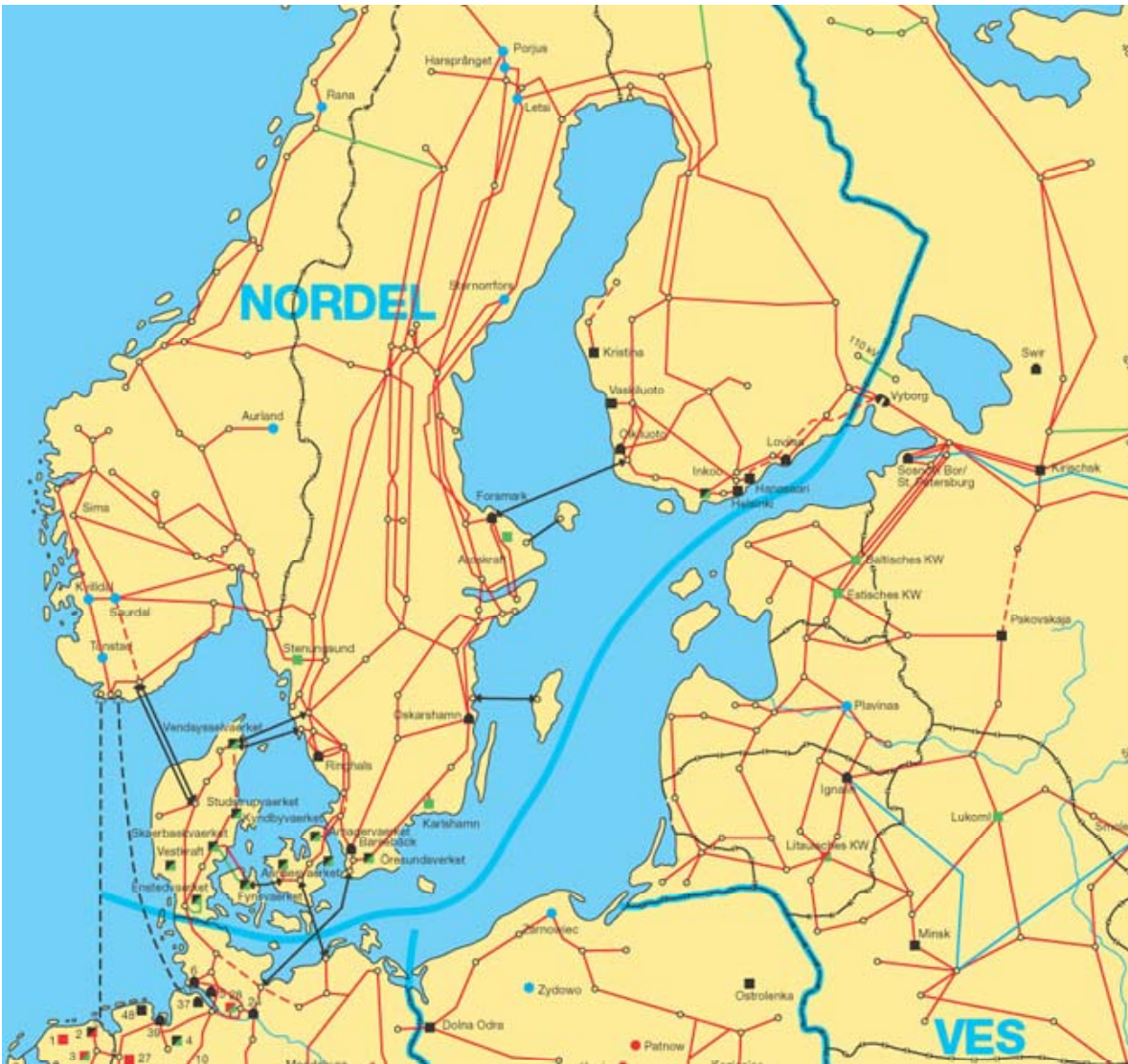
Fig. 5: Electrical transmission network in the countries around the Baltic Sea. The red lines indicate the 380kV grid, the blue lines the 300kV grid and the green lines the 220kV grid. The small black dots on the lines indicate grid nodes. The black and blue rectangles and the larger black dots indicate power plants [Ref 49].
