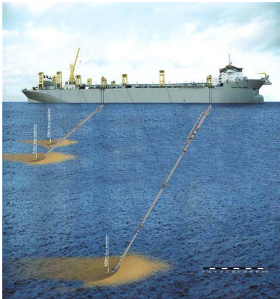
Fig. 17: A large suction hopper dredger, excavating sediment at different sea depths. The excavated sediment is pumped into the ship's cargo bay and is later deposited in a different sea area.
