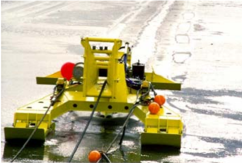
Fig. 21: Burial sledge for laying cable in shallow water and mud flats.
