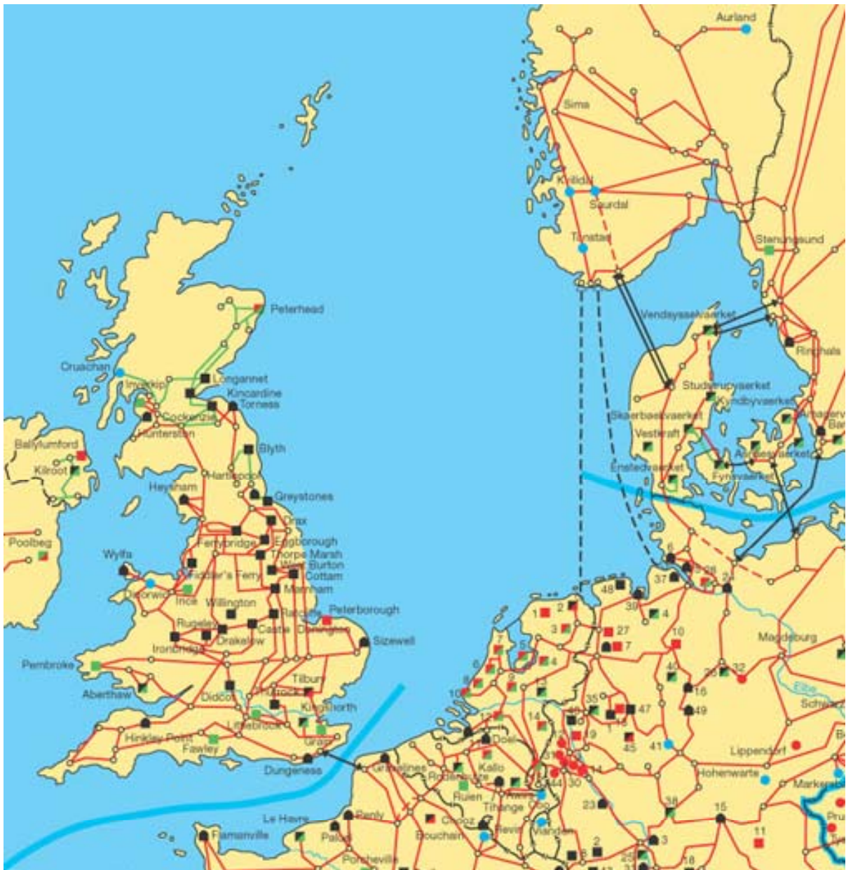
Fig. 4: Electrical transport network in the countries around the North Sea [Ref 49]. The red lines indicate 380kV grid. The small dots on the lines (open circles) indicate network nodes. The black and coloured squares and the larger coloured dots indicate power plants.
