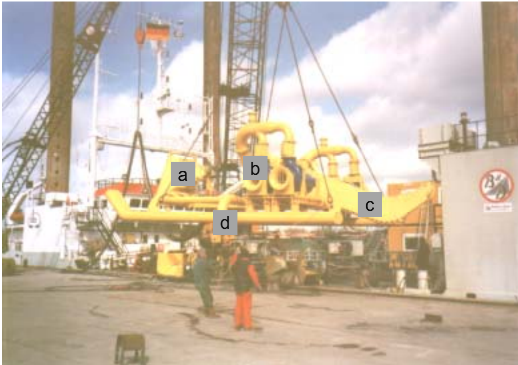
Fig. 20: Burial sledge for submarine cables (a: cable inlet; b: pumps; c: sword with nozzles, able to be lowered to different depth; d: sledge runners).
